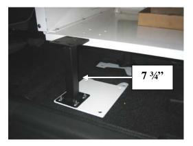
Sub-assemble mounting leg to mounting plate using <sup>1</sup>/<sub>4</sub>" x <sup>3</sup>/<sub>4</sub>" carriage bolts and serrated nuts. Set mounting leg assembly to 7 <sup>3</sup>/<sub>4</sub>"
